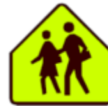
WC-1 (School Area)
