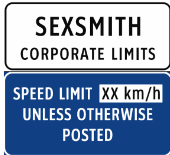
FIGURE 30. ALBERTA RECOMMENDED COMMUNITY SPEED LIMIT INFORMATION SIGN
